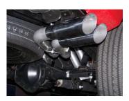
7. Attach tailpipes together with bolt kit #H. Driver side tab should be on the bottom.
