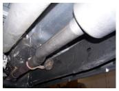
**2.** Insert muffler assembly #A into headpipe head pipe and attach with clamp #B. DO NOT TIGHTEN Use a jack stand to support the muffler assembly.
