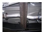
**3.** Bolt head pipe #A onto your existing stock front pipe re-using stock nuts/bolts. Use a jack stand to support the converter. Insert welded hanger into rubber grommet.DO NOT TIGHTEN.
