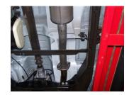
**4.** Install muffler #B onto head pipe #A 1½"-2". Use a jack stand to support the muffler. Use clamp #E to secure the muffler to the headpipe. Do not tighten.
