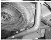
Install the Driver side over-axle tailpipe #D into the muffler 1-1/2" to 2". Then insert the welded hanger into the rubber grommet. Use clamp #H to secure it to the muffler. **Do Not Tighten at this Time!**
