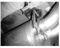
Install rear muffler hanger #H. Onto driver side outlet of the muffler, insert hanger into rubber grommet.
