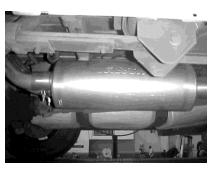
Install muffler #B onto head-pipe #A 1-1/2" to 2" with the louvers in the muffler facing towards the converter. Use a jack stand to support the muffler. Use Clamp #F to secure the muffler to the head-pipe. **Do Not Tighten at this Time!**
