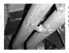
USING BOLT KIT #J AND ATTACH BOTH TAILPIPES. THE PASSENGER SIDE MOUNTING BRACKET WILL BE POSITIONED UNDERNEATH THE DRIVER SIDE.
