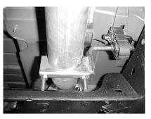
INSTALL HANGER # F ONTO HEADPIPE # A, AND INSERT WELDED HANGER INTO RUBBER GROMMET. DO NOT TIGHTEN.
