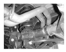
SLIP TAILPIPE #C INTO THE DRIVER SIDE OUTLET NO MORE THEN 2" AND NO LESS THEN 1". USE HANGER # E TO TIGHTEN THE CONNECTION AT THE MUFFLER OUTLET. DO NOT TIGHTEN
