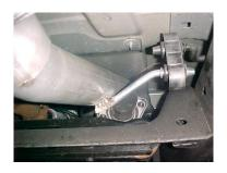
INSTALL HEAD PIPE # A ONTO YOUR EXISTING STOCK FRONT PIPE. INSERT WELDED HANGER INTO RUBBER GROMMET. YOU WILL BE USING THE FACTORY HARDWARE.
