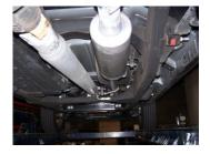
by unbolting it at the flange located in front of the muffler. Disengage the welded hangers from the OEM rubber grommets. Use WD-40 to aid in this process. Do not damage stock nuts and bolts or remove the rubber grommets as you will re-use them to mount your new system. Now, cut off tailpipe and remove system.
