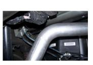
7. Slide driver side tailpipe #D into muffler 11/2"-2" and secure with clamp #F. Do not tighten. Insert welded hangers into rubber grommets.
