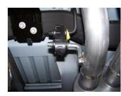
7. Install driver's side rear hanger #M onto side of frame as seen in picture. Secure bolt kit #0 to frame. Use grommet #L and clamp hanger #N. This clamp also holds exit pipe to tailpipe.
