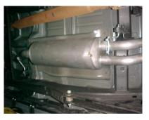
INSTALL MUFFLER # B ONTO HEAD PIPE 1-1/2"-2" WITH THE LOUVERS FACING TOWARDS THE CONVERTER. USE A JACK STAND TO SUPPORT THE MUFFLER. USE CLAMP # F TO SECURE THE MUFFLER TO THE HEADPIPE. DO NOT TIGHTEN.
