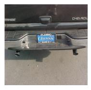
INSTALL STAINLESS TIPS. CLAMP DOWN. WHEN YOU HAVE EVERYTHING IN PLACE, FIRMLY TIGHTEN ALL BOLTS AND CLAMPS DOWN SECURELY. TO CLEAN TIPS, USE A STAINLESS STEEL CLEANER AND A SCOTCH BRITE PAD.
