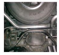
INSTALL THE PASSENGER SIDE OVERAXLE TAILPIPE #D TO THE MUFFLER 1-1/2"-2". USE CLAMP # G TO SECURE TAILPIPE TO MUFFLER. DO NOT TIGHTEN.
