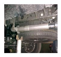
INSTALL EXIT PIPES # E. USE CLAMPS # G TO SECURE TO THE TAILPIPES. DO NOT TIGHTEN.
