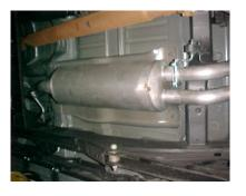
INSTALL MUFFLER # B ONTO HEAD PIPE 1-1/2"-2" WITH THE LOUVERS FACING TOWARDS THE CONVERTER. USE A JACK STAND TO SUPPORT THE MUFFLER. USE CLAMP # G TO SECURE THE MUFFLER TO THE HEADPIPE. DO NOT TIGHTEN.
