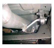
INSTALL HEAD PIPE # A ONTO YOUR EXISTING STOCK FRONT PIPE. INSERT WELDED HANGER INTO RUBBER GROMMET.
