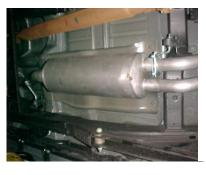
INSTALL MUFFLER # B ONTO HEAD PIPE 1-1/2"-2" WITH THE LOUVERS FACING TOWARDS THE CONVERTER. USE A JACK STAND TO SUPPORT THE MUFFLER. USE CLAMP # G TO SECURE THE MUFFLER TO THE HEADPIPE. DO NOT TIGHTEN.
