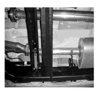
LAY OUT THE GIBSON EXHAUST ON THE FLOOR AND COMPARE PART #'S TO THE DRAWING. TO REMOVE STOCK EXHAUST, REMOVE IT FROM THE 2-BOLT FLANGE LOCATED IN FRONT OF THE MUFFLER. DO NOT DISGUARD FACTORY HARDWARE YOU WILL RE-USE IT. LEAVE ALL RUBBER GROMMETS IN PLACE. USE WD-40 TO AID IN REMOVAL OF EXHAUST AND THE RUBBER GROMMETS.
