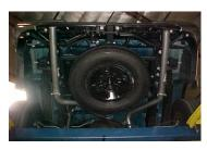
Now go back and tighten all clamps, nuts and bolts. Start from the front and work back.
