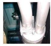
Next, install rear muffler hanger #H onto drivers side muffler outlet insert hanger into rubber grommet. Do not tighten.
