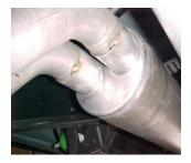
Install muffler # C onto head pipes 1-1/2" to 2" with the louvers facing towards the converter. Use a jack stand to support the muffler. Use clamps #G to the secure the muffler to the head pipes. Do not tighten. Outlets will be on the bottom.
