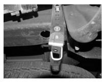
INSTALL METAL HANGERS #H INTO HOLES LOCATED APPROX. 16" FROM THE REAR OF THE FRAME. METAL HANGERS ARE MOUNTED ON THE OUTSIDE OF FRAME. USE HARDWARE KIT #I.. THE BOLT AND WASHER WILL GO INTO THE 3RD HOLE FROM THE TOP OF THE HANGER.
