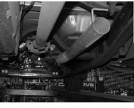
INSTALL MUFFLER #B ONTO HEADPIPE AT LEAST 1 1/2" TO 2". USE CLAMP #F TO SECURE MUFFLER TO HEADPIPE. DO NOT TIGHTEN. USE A JACK STAND TO SUPPORT THE MUFFLER. OUTLETS
