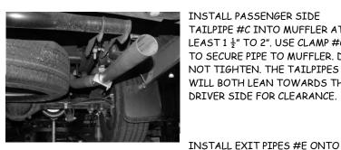
INSTALL PASSENGER SIDE TAILPIPE #C INTO MUFFLER AT LEAST 1 ½" TO 2". USE CLAMP #G TO SECURE PIPE TO MUFFLER. DO NOT TIGHTEN. THE TAILPIPES WILL BOTH LEAN TOWARDS THE DRIVER SIDE FOR CLEARANCE.
