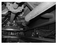
TO REMOVE STOCK EXHAUST UNBOLT IT FROM THE FLANGE LOCATED JUST BEHIND THE FACTORY Y-PIPE. YOU WILL RE-USE YOUR FACTORY BOLTS FROM FLANGE, NOW, CUT OFF YOUR STOCK TAILPIPE JUST BEHIND THE MUFFLER AND REMOVE. LEAVE ALL RUBBER GROMMETS ON THE HANGER. USF WD-40 TO AID IN REMOVAL OF THE EXHAUST AND HANGERS.
