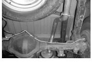
Slip the over axle tailpipes #C, #D into the outlets of the muffler no more then 1- 1/2" to 2" and attach clamp #G to passenger side and clamp hanger # I to driver side tailpipe.
