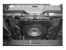
Install exit pipes # E onto the over axle pipes and attach with clamp #G. You may need to cut the exit pipes to your preference. Rotate all pipes until you have a minimum of a 1" clearance on all pipes. Use zip ties for brake lines. Tighten all clamps, flanges, and bolts firmly. Install stainless steel tips. Use zip ties for brake and fuel lines.
