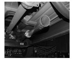
INSTALL HEADPIPE #B ONTO STOCK FLANGE, USE STOCK 15MM NUTS TO SECURE IT. DO NOT TIGHTEN, JUST MAKE SNUG.
