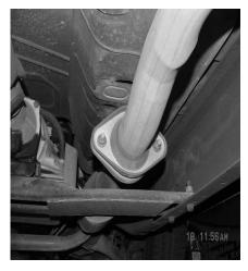
TO REMOVE EXHAUST- UNBOLT THE 2 BOLT FLANGE LOCATED BEHIND THE CATALITIC CONVERTER. SAVE STOCK NUTS AND BOLTS FOR YOU WILL REUSE THEM. NOW CUT OFF YOUR STOCK TAILPIPE JUST BEHIND THE MUFFLER AND REMOVE. LEAVE ALL RUBBER GROMMETS ON THE HANGER. USE WD-40 TO AID IN THE REMOVAL OF THE EXHAUST AND HANGERS.
