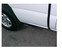
INSTALL YOUR STAINLESS TIPS, NOW TIGHTEN ALL NUTS, BOLTS, AND CLAMPS. TO CLEAN YOUR STAINLESS TIPS USE A SCOTT BRITE PAD AND ANY STAINLESS STEEL OR ALUMINUM CLEANER.
