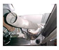
INSTALL HEADPIPE #A ONTO YOUR EXISTING STOCK 2-BOLT FLANGE. USE YOUR STOCK HARDWARE TO SECURE. DO NOT TIGHTEN. USE A JACK STAND TO SUPPORT THE CONVERTER.
