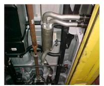
INSTALL MUFFLER ASSEMBLY #B ONTO HEADPIPE #A. SLIDE WELDED HANGERS INTO RUBBER GROMMETS. USE CLAMP #C TO SECURE MUFFLER ASSEMBLY TO HEADPIPE. DO NOT TIGHTEN.
