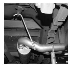
SLIDE MUFFLER ASSEMBLY ONTO HEADPIPE 1 1/2" TO 2". INSERT WELDED HANGER INTO RUBBER GROMMET ON DRIVERSIDE USING CLAMP #C TO SECURE MUFFLER TO HEADPIPE. DO NOT TIGHTEN.
