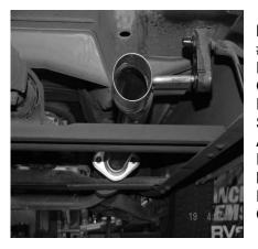
BOLT HEADPIPE #A TO STOCK FLANGE USING GASKET # F AND RE-USING STOCK NUTS AND BOLTS. INSERT WELDED HANGER INTO RUBBER GROMMETS.
