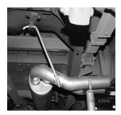
SLIDE MUFFLER ASSEMBLY #B ONTO HEADPIPE 1-1/2" TO 2". INSERT WELDED HANGER INTO RUBBER GROMMET ON DRIVERSIDE USING CLAMP #C TO SECURE MUFFLER TO HEADPIPE. DO NOT TIGHTEN. USE A JACK STAND TO SUPPORT MUFFLER.
