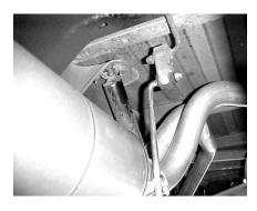
INSTALL REAR MUFFLER HANGER #J ONTO DRIVERS SIDE MUFFLER OUTLET. INSERT THE WELDED HANGER INTO RUBBER GROMMET. DO NOT TIGHTEN. INSTALL DRIVERSIDE TAILPIPE #D INTO MUFFLER 1-1/2" TO 2". THIS PIPE GOES BETWEEN THE SHOCK & FRAME. SLIDE CLAMP #H OVER PIPE AND CONNECT IT TO THE HANGER#I. THIS WILL HOLD UP THE TATLPTPE.
