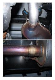
1. To remove the stock exhaust remove it from in front of the stock muffler. Disengage the welded hangers using WD-40 from the OEM rubber grommets. Do not damage or remove the rubber grommets as you will re-use them to mount your new system. Now, cut off tailpipe and remove exhaust.
