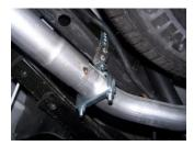
**7.** Install exit pipes #E, use clamps #G to secure to tailpipes. DO NOT TIGHTEN.
