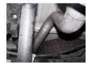
**4.** Install passenger side tailpipe #C into muffler 1½-2". Use clamp #G to secure tailpipe to muffler. DO NOT TIGHTEN. Insert welded hanger into rubber grommet.
