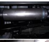
**3.** Install muffler #B onto head pipe #A 1½"-2" with the louvers facing towards the converter. Use a jack stand to support the muffler. Use clamp #G to secure the muffler to the headpipe. Slide band clamp onto muffler and insert welded hangers into rubber grommets. Attach with bolt kit #J. DO NOT TIGHTEN. Muffler inlet is looking into the louvers.
