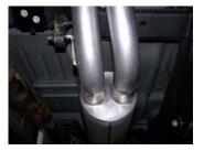
4. Install muffler #B onto headpipe 1.5-2" with the louvers facing towards the converter. Use a jack stand to support the muffler. Use clamp #G to secure the muffler to the headpipe. Do not tighten. Muffler inlet is looking into louvers.
