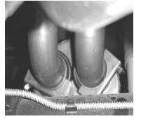
INSTALL TAILPIPES#C, D USE CLAMP#G ON THE PASSENGER SIDE AND HANGER #I ON THE DRIVER SIDE, INSERT WELDED HANGER INTO RUBBER GROMMET. USE BOLT KIT#H TO CONNECT BOTH THE TAILPIPES TOGETHER.
