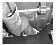
NEXT, CONNECT HEADPIPE#A TO THE STOCK FLANGE. RE-USE STOCK NUTS AND GASKET # J.
