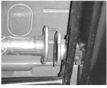
AFTER CUTTING THE TAILPIPE, UNBOLT THE STOCK HEADPIPE AND REMOVE THE WHOLE SYSTEM.LEAVE ALL RUBBER GROMMETS IN PLACE. YOU WILL RE-USE THE FACTORY BOLTS.BEFORE REMOVING MAKE SURE YOU SUPPORT THE CATALITIC CONVERTER IN THE STOCK POSITION.
