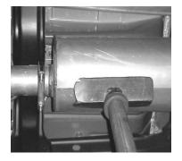
INSTALL MUFFLER # B ONTO HEADPIPE #A 1 1/2" TO 2"". THE INLET WILL BE AT APPROXIMATELY 6 O'CLOCK. CONNECT THE MUFFLER TO HEADPIPE#A USING CLAMP#F. INSERT WELDED HANGER INTO RUBBER GROMMET.
