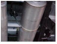
ONTO HEADPIPE 1-1/2" TO 2". USE CLAMP #H TO SECURE THE MUFFLER TO THE HEADPIPE, DO NOT TIGHTEN. SLIDE BAND CLAMP #I ONTO THE MUFFLER AND INSERT THE WELDED HANGER INTO THE RUBBER GROMMET AND ATTACH WITH BOLT KIT #J.
