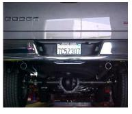
**INSTALL THE EXIT** PIPES #E ONTO THE TAILPIPES USING CLAMPS #G. ROLL THE PIPES UNTIL YOU HAVE THEM AT THE ANGLE YOU DESIRE.
