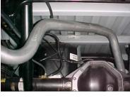
**INSTALL DRIVER SIDE** TAILPIPE #D INTO MUFFLER 1-1/2" TO 2" AND USE CLAMP #G TO SECURE THE MUFFLER. DO NOT TIGHTEN. USE CLAMP #G TO HOLD PIPE UP TO THE HANGER #F. DO NOT TIGHTEN.
