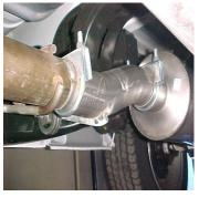
INSTALL HEADPIPE #A, YOU WILL NEED TO LINE UP THE TWO NOTCHES. **INSERT HANGER INTO** RUBBER GROMMET, DO NOT TIGHTEN. USE CLAMP #M TO SECURE HEADPIPE TO YOUR STOCK PIPE. DO
