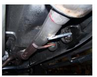
INSTALL HEADPIPE #A ONTO YOUR EXISTING STOCK FRONT PIPE AND SECURE WITH CLAMP #K. USE A JACKSTAND TO SUPPORT THE CONVERTER. INSERT WELDED HANGER INTO RUBBER GROMMET. DO NOT TIGHTEN.
