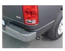
INSTALL THE STAINLESS TIPS. NOW GO BACK AND TIGHTEN ALL CLAMPS, NUTS AND BOLTS STARTING FROM THE FRONT AND WORKING BACK. TO CLEAN TIPS USE ANY STAINLESS CLEANER.
