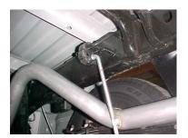
INSTALL HEADPIPE #A, YOU WILL NEED TO LINE UP THE TWO NOTCHES. USE HEADPIPE HANGER #K TO SECURE PIPES TOGETHER. INSERT HANGER INTO RUBBER GROMMET. DO NOT TIGHTEN.
