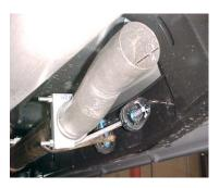
INSTALL HEADPIPE #A ONTO YOUR EXISTING STOCK FRONT PIPE AND SECURE WITH CLAMP #K. USE A JACKSTAND TO SUPPORT THE CONVERTER. INSERT WELDED HANGER INTO RUBBER GROMMET. DO NOT TIGHTEN.
