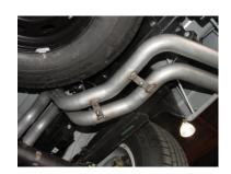
INSTALL PASSENGER SIDE TAILPIPE #D INTO MUFFLER AND ATTACH USING CLAMP #F. INSERT WELDED HANGER INTO RUBBER GROMMET. DO NOT TIGHTEN. USE BOLT KIT #I TO ATTACH THE TAILPIPES TOGETHER. DO NOT TIGHTEN. PASSENGER SIDE TABS ON TAILPIPE WILL BE ON TOP OF DRIVER SIDE TABS.
