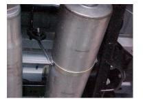
INSTALL MUFFLER #B ONTO HEADPIPE 1-1/2" TO 2". USE CLAMP #H TO SECURE THE MUFFLER TO THE HEADPIPE. DO NOT TIGHTEN. SLIDE BAND CLAMP #I ONTO THE MUFFLER AND INSERT THE WELDED HANGER INTO THE RUBBER GROMMET. ATTACH WITH BOLT KIT #L.
