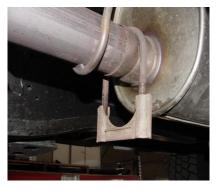
TO REMOVE STOCK EXHAUST UNCLAMP IT FROM THE CLAMP LOCATED JUST IN FRONT OF YOUR STOCK MUFFLER. YOU MAY NEED TO HEAT IT UP WITH A TORCH TO REMOVE IT. NOW CUT OFF YOUR STOCK TAILPIPE JUST BEHIND THE MUFFLER AND REMOVE.LEAVE ALL RUBBER GROMMETS ON THE HANGER, USE WD-40 TO AID IN REMOVAL OF EXHAUST AND HANGERS.
