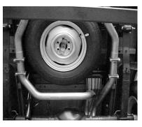
ATTACH EXIT PIPES # D
