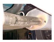
Lay out the exhaust on the floor so it looks like the drawing and compare parts with manual. **To remove the stock exhaust cut 13" just in front of the muffler.** Leave all rubber
