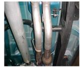
Install driverside headpipe #B. Then install headpipe #A and insert welded hanger into rubber grommet. Secure both pipes with clamp #H. Do not tighten.
