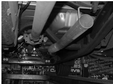
INSTALL PASSENGER SIDE TAILPIPE #C INTO MUFFLER AT LEAST 1 1/2" TO 2". USE CLAMP #G TO SECURE PIPE TO MUFFLER. DO NOT TIGHTEN. THE TAILPIPES THEY WILL BOTH LEAN TOWARDS THE DRIVER SIDE LOOKING FROM THE REAR OF THE VEHICLE - THIS TAILPIPE IS AT APPX. 11 O'CLOCK.
