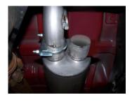
5. Install driver side over axle tailpipe #C into muffler 1.5-2". Use clamp #G to secure tailpipe to muffler, DO NOT TIGHTEN.
