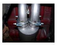
7. Install passenger side over axle tailpipe #E into muffler 1.5-2". Use clamp #G to secure. DO NOT TIGHTEN. Insert welded hanger into
