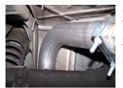
6. Install muffler assembly #B onto head pipe. Insert hangers into rubber grommets. Use a iack stand to support the muffler. Use clamp #G to secure the muffler to the head pipe. Do not tighten.
