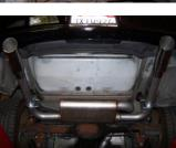
7. Next, install the exit pipes #C. Use clamp #E to secure tail pipes.
