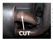
2. To remove the stock exhaust, cut off your stock over axle tailpipe just at the muffler. Then remove hangers from rubber grommets and remove muffler assembly.
