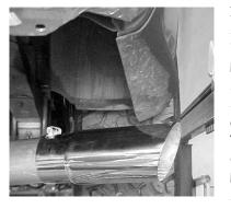
INSTALL THE STAINLESS STEEL TIP TO YOUR DESIRED LOOK. USE ANY ALUMINUM OR STAINLESS STEEL CLEANER TO POLISH YOUR TIP.TURN VEHICLE ON AND CHECK FOR LEAKS. NOW TIGHTEN ALL CLAMPS AND MAKE SURE ALL HANGERS ARE IN THE CORRECT PLACE.
