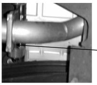
INSTALL OVERAXLE #C INTO THE OUTLET OF THE MUFFLER NO LESS THEN 1-1/2" AND NO MORE THEN 2". USING CLAMP #H. INSERT WELDED HANGER INTO RUBBER GROMMET. SLIP TURNOUT PIPE #D ONTO OVERAXLE PIPE AND INSTALL WITH CLAMP #F. DO NOT TIGHTEN.
