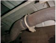
DRAWING. TO REMOVE YOUR FACTORY EXHAUST REMOVE IT FROM THE CLAMP LOCATED IN FRONT OF THE MUFFLER. YOU MAY NEED TO HEAT IT UP FOR EASIER REMOVAL. USE WD-40 TO AID YOU IN REMOVING HANGERS LEAVE ALL RUBBER GROMMETS IN
