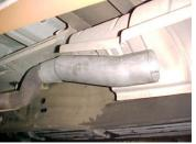
INSTALL HEADPIPE #A ONTO FACTORY PIPE. LINE UP NOTCH. USE CLAMP #G TO SECURE. DO NOT TIGHTEN.
