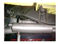
SLIDE MUFFLER#C ONTO THE HEADPIPE 1 ½" TO 2". THE MUFFLER INLET IS LOOKING INTO THE LOUVERS. USE JACK STAND TO SUPPORT THE MUFFLER. ATTACH CLAMP #G AT THE INLET OF THE MUFFLER. THE MUFFLER OUTLET SHOULD BE POSITIONED AT ABOUT 12 O'CLOCK. DO NOT TIGHTEN
