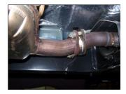
1. To remove the stock exhaust, un-bolt it from the 2-bolt flange. Save stock bolts they will be reused. Disengage the welded hangers using WD-40 from the OEM rubber grommets. Do not damage or remove the rubber grommets as you will re-use them to mount your new system. Now, cut off tailpipe and remove.
