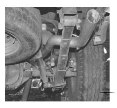
INSTALL OVERAXLE TAILPIPE #B INTO MUFFLER. INSERT WELDED HANGER INTO FACTORY RUBBER GROMMET. CLAMP DOWN WITH HANGER #D TO MUFFLER. DO NOT TIGHTEN
