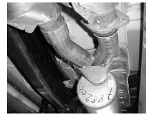
INSTALL MUFFLER ASSEMBLY #A. REUSE DRIVERSIDE HEADPIPE GASKET & APPLY SMALL AMOUNT OF HI-TEMP GASKET SEALER. BOLT DRIVERSIDE FLANGE & REUSE FACTORY BOLTS. ATTACH THE PASSENGER SIDE HEADPIPE USING CLAMP #E. DO NOT TIGHTEN
