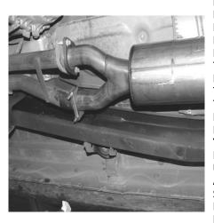
LAYOUT THE GIBSON EXHAUST AND COMPARE PART NUMBERS TO THE PIPE NUMBERS. FOR EASY REMOVAL, CUT THE STOCK TAILPIPE BEHIND THE MUFFLER AND ALSO BEHIND THE AXLE. NOW UNBOLT THE STOCK FLANGE AND REMOVE THE STOCK MUFFLER. DO NOT DAMAGE THE FACTORY GASKET **BECAUSE YOU WILL RE-USE IT.** INSTALL MUFFLER ASSEMBLY#A ONTO THE STOCK FLANGE REUSING THE FACTORY GASKET AND BOLTS. SECURE PASSENGER SIDE HEADPIPE WITH CLAMP #E. DO NOT TIGHTEN!!
