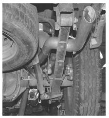
NOW GO BACK AND TIGHTEN THE FLANGE AT THE CATALYTIC CONVERTER AND HANGER **#D. MAKE SURE** EVERYTHING IS TIGHT. ALSO, MAKE SURE YOU HAVE AT LEAST 1" CLEARANCE ON ALL PIPES FROM ALL RUBBER BRAKE LINES, SHOCK BOOTS, TIRES, ETC. YOU MAY NEED TO LOOSEN THE SPARE TIRE AND PUSH IT TO THE DRIVER SIDE FOR CLEARANCE PURPOSES.
