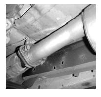
SLIDE FLANGE #D ONTO HEADPIPE #A AND BOLT TO FACTORY HEADPIPE REUSING FACTORY NUTS & BOLTS. (DO NOT TIGHTEN), OUTLET OF HEADPIPE SHOULD BE AT ABOUT 1'OCLOCK. SLIDE MUFFLER #B ONTO THE HEADPIPE NO MORE THEN 2" AND NO LESS THEN 1" ON THE INLET OF THE MUFFLER AND CLAMP WITH #G. MUFFLER INLET IS LOOKING INTO THE LOUVERS.
