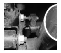
SLIP THE OVERAXLE PIPE #C THROUGH THE LEAF SPRING IN BETWEEN THE SHOCK AND THE SWAY-BAR AND INTO THE MUFFLER AT LEAST 1 ½" NO MORE THAN 2" USE HANGER #E TO CLAMP PIPE TO MUFFLER.
