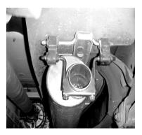
ONCE THE MUFFLER AND HEADPIPE ARE INSTALLED ROTATE THE MUFFLER AND HEADPIPE UNTIL MUFFLER OUTLET IS POSITIONED AT 3 O'CLOCK AND SITTING LEVEL UNDERNEATH THE VEHICLE. INSTALL THE O.E. HANGER #E ONTO OUTLET OF MUFFLER AND INSERT WELDED HANGERS INTO DI IRRED GOOMMET
