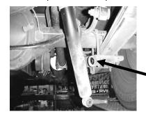
FOR AN EASIER INSTALLATION OF THE OVERAXLE PIPE DISCONNECT THE LOWER REAR SHOCK MOUNT.
