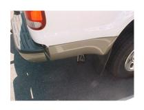
**5.** NOW INSTALL YOUR STAINLESS STEEL TIP. USE ANY ALUMINUM OR STAINLESS CLEANER TO POLISH YOUR TIP. THEN TIGHTEN ALL CLAMPS AND HANGERS.
