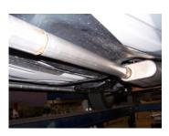
5. Install extension pipe #C onto muffler outlet. Use clamp #H to secure the pipe to the muffler. Insert welded hanger into rubber grommet.
