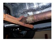
2. To remove the stock exhaust, unclamp it at the connection in front of the stock muffler. Disengage the welded hangers from the rubber grommets using WD-40 to aid in this process. Do not damage or remove the rubber grommets as you will re-use them to mount the new system.
