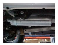
Install muffler # B onto head pipe # A 1-1/2" to 2" with the louvers facing towards the converter. Use a jack stand to support the muffler. Use clamp # G to secure the muffler to the head pipe. Do not tighten. Muffler inlet is looking into the louvers.
