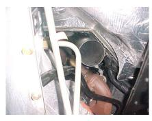
INSTALL PIPE #J ONTO TURBO USING YOUR STOCK CLAMP. DO NOT TIGHTEN.
