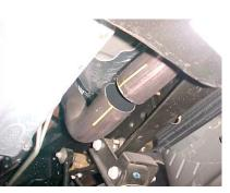
TO INSTALL YOUR GIBSON DOWN PIPE YOU NEED TO REMOVE YOUR STOCK EXHAUST. REMOVE THE STOCK EXHAUST FROM THE CLAMP LOCATED JUST BEHIND THE CATALYTIC CONVERTER. CUT OFF YOUR STOCK TAILPIPE FOR EASIER REMOVAL. LEAVE ALL RUBBER GROMMETS IN PLACE. USE WD-40 TO AID IN REMOVAL OF EXHAUST AND HANGER. AFTER YOUR STOCK EXHAUST IS REMOVED YOU NEED TO REMOVE THE CATALYTIC **CONVERTER FROM THE 2-**BOLT FLANGE.
