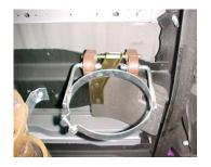
Install band clamp # F into rubber grommets located iust above the axle. Do not tighten. And attach with bolt kit # I.
