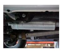
Install muffler # B onto head pipe # A 1-1/2" to 2" with the louvers facing towards the converter. Use a jack stand to support the muffler. Use clamp # G to secure the muffler to the head pipe. Do not tighten. Muffler inlet is looking into the louvers.
