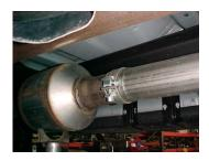
Lav out the exhaust on the floor so it looks like the drawing and compare parts with manual. To remove the stock exhaust remove it from the clamp located just behind the catalytic converter. Cut off your stock tailpipe for easier removal. Leave all rubber grommets in place. Use WD-40 to aid in removal of exhaust and hangers.
