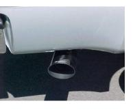
Install the over axle tailpipe # C into the muffler 1-1/2" to 2". Secure to the muffler using clamp # G Do not tighten.
