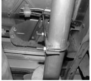
TAILPIPE #C INTO THE MUFFLER NO MORE THAN 1 ½" TO 2". INSERT WELDED HANGER INTO RUBBER GROMMET. USE CLAMP #G TO ATTACH T-HANGER # H ONTO OVERAXLE TAILPIPE AND INSERT INTO RUBBER GROMMET. THE HANGER TOWARDS THE DRIVERSIDE. MAKE SURE YOU HAVE **EQUAL SPACE BETWEEN** SHOCK AND SPARE TIRE. THE SPARE TIRE MAY NEED TO BE LOOSENED AND PUSH TO THE DRIVER SIDE AND THEN ROTATE TO GAIN CLEARANCE. FX4 MODELS MAY NEED TO REMOVE RIGHT REAR SHOCK BOOT
