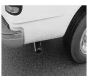
**INSTALL THE STAINLESS** STEEL TIP. USE ANY ALUMINUM OR STAINLESS STEEL CLEANER TO POLISH TIP. NOW TIGHTEN ALL CLAMPS, BOLTS AND HANGERS.
